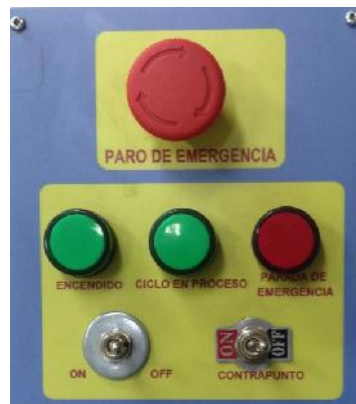
Figura 62 Tablero de control principal del torno NCL2000.
