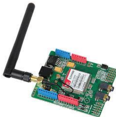
Figura 8 Arduino GSM Shield. ( Electronics )
