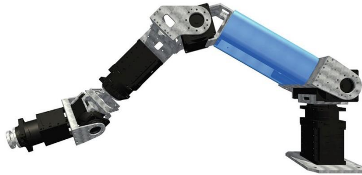
Fig. 6. Arm Robotic 6DOF developed in SolidWorks
