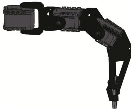
Fig. 3. Hexapod robot: assembly of an extremity
