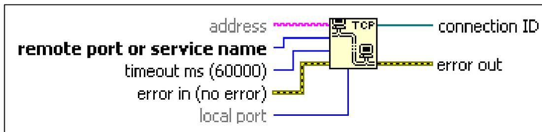
**Figura N° 57: TCP Open Connection Function**
