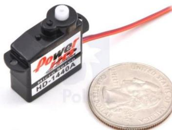
**Figura 52 Mini Servo Power HD 1440A**
