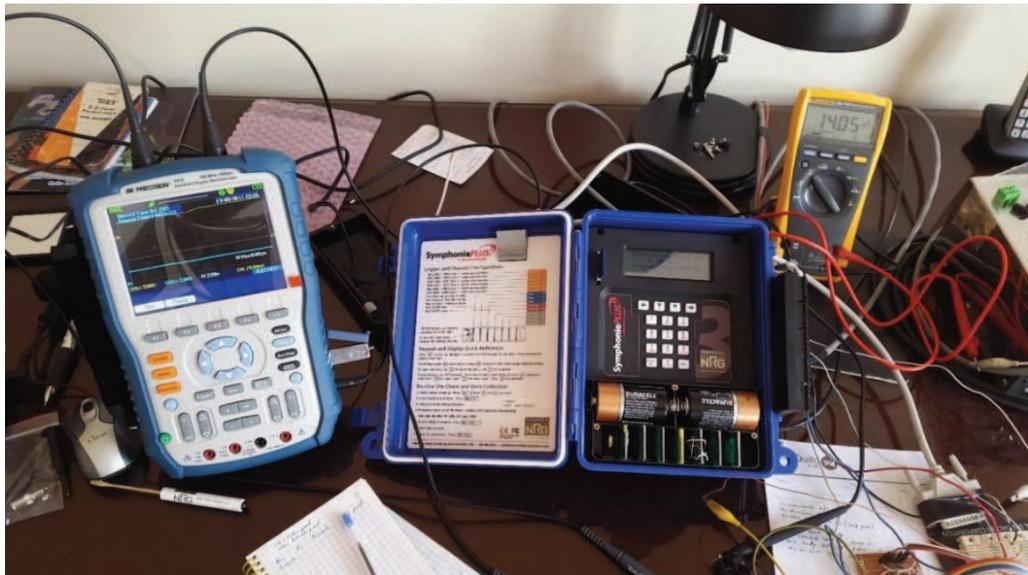
**Figura 92.** Osciloscopio digital BK 5100, 100 Mhz
