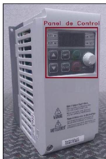
Figura 92. Panel de control VDF
