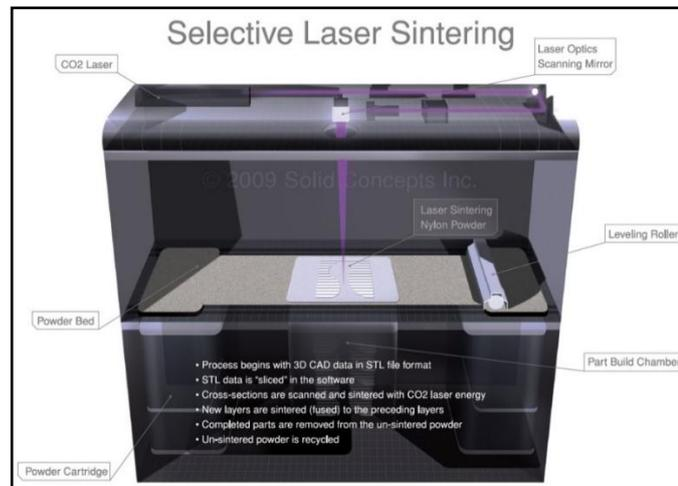
**FIGURA 6:** TECNOLOGÍA SLS (SELECTIVE LASER SINTERING)
