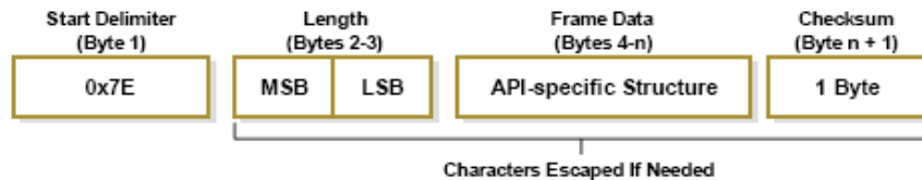
Figure 4-07. UART Data Frame Structure - with escape control characters:
