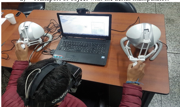
b) Handling of the aerial manipulator with the Haptic device.
