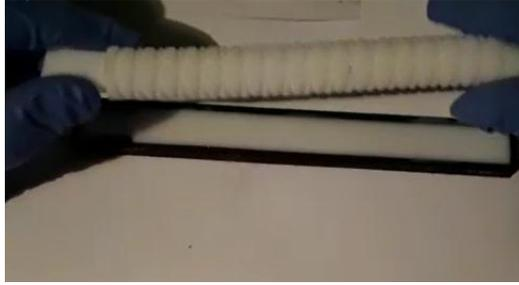
**Figura 60.** Unión de capas extensible e inextensible
