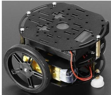
*Figura 25.* Mini 3-layer round robot de Adafruit.
