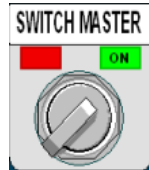
Figura. 4.17 Selector Switch Master Modo manual
