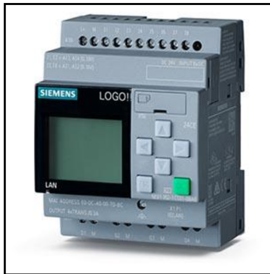
Figura 10. PLC compacto de SIEMENS LOGO! 8 Basic.
