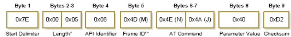
Figure 4-12. Example: API frames when modifying the NJ parameter value of the module.
