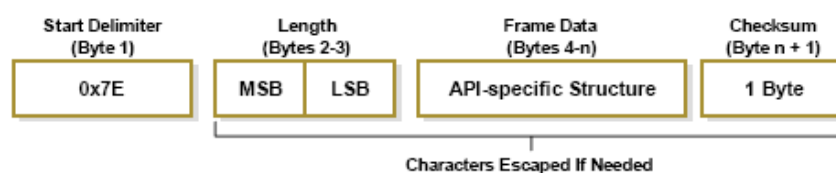
Figure 4-07. UART Data Frame Structure - with escape control characters:
