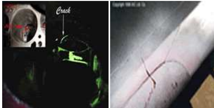
Figura 2.5 Ensayos de Líquidos Penetrantes .( General Electric Inspection technologies, Penetrant Testing, 2004 )
