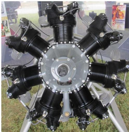
**Figura 5 Motor radial**
