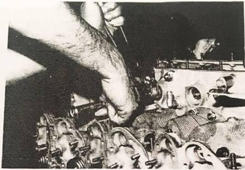
FIGURE 72-60-10. INSTALLING PUSHROD HOUSING.
