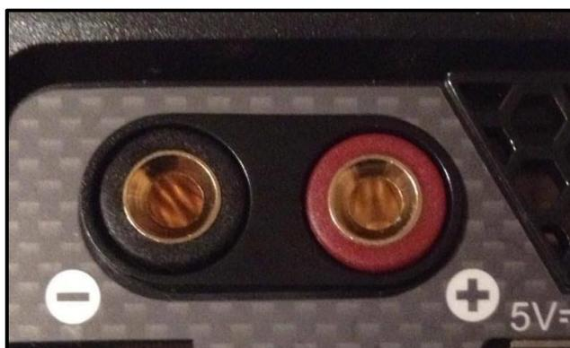
**Figura 26** Conector de salida, conector Banana de 4mm
