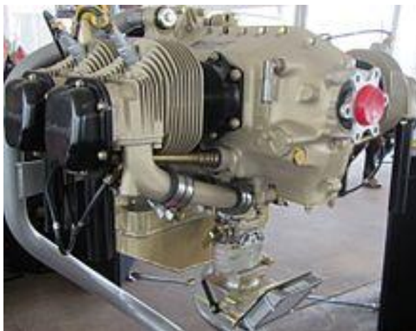
Figura 3 Motor Teledyne Continental O-200 Fuente : (Zenith Aircraft Company , 2010)
