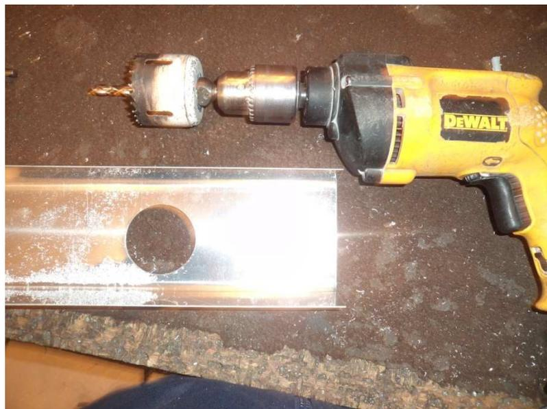
**Figura 3.19** Floor beam perforado
