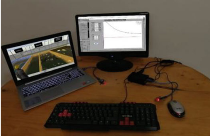
Fig. 48.8 Implementation of the hardware-in-the-loop technique
