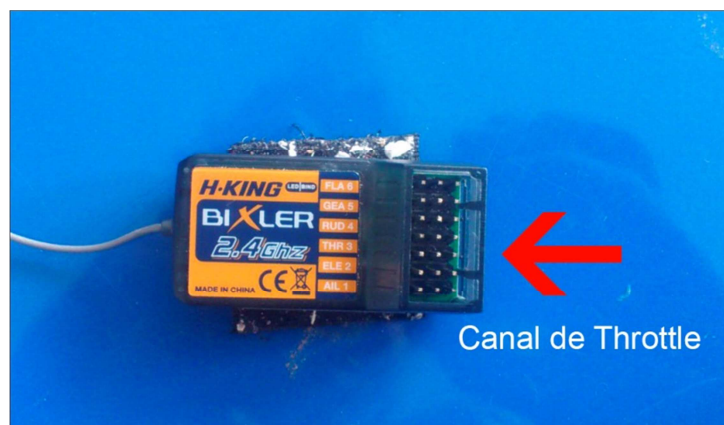
Foto 3. 12. Canal 3 del receptor (Throttle)
