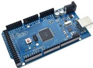
A blue Arduino Mega microcontroller board with various components like a USB Type-B port, a DC power jack, and several integrated circuits.  |
