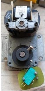
A photograph of an AC motor assembly, showing a black cylindrical motor mounted on a metal base with a green terminal block.               |
