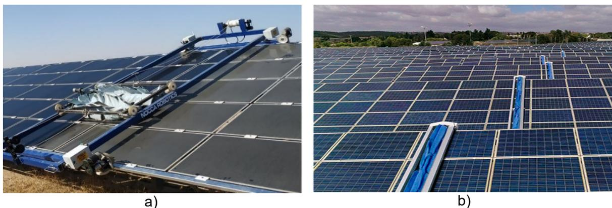
Nota. a) NOCCA S100 (Cepillo Horizontal) y b) AirTouch 3.0 (Cepillo Vertical). Adaptado de “A review on cleaning mechanism of solar photovoltaic panel”, por (Patil et al., 2017).
