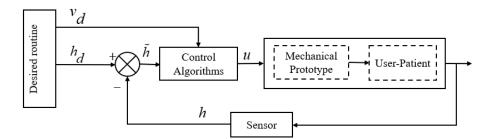
Fig. 2. Autonomous control of rehabilitation system.
