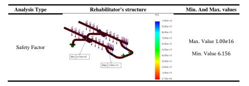
During the analysis, a force of 177 [N] was applied. As a result, it is determined that the rehabilitator does not experience stresses that exceed its elastic limit. The maximum value of the displacement of the rehabilitator is 0.317 [mm]. In addition, it is observed that there is no unitary deformation. Finally, it is noted that the safety factor mechanically qualifies the device as safe.
