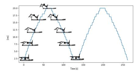
**Fig. 10**. Motion reconstruction based on real data. The generated graph is shown with small distortions due to the sampling time, which is 500ms, sufficient time according to the capacity of the microprocessor.
