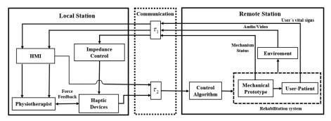
Fig. 5. Bilateral telerehabilitation scheme.
