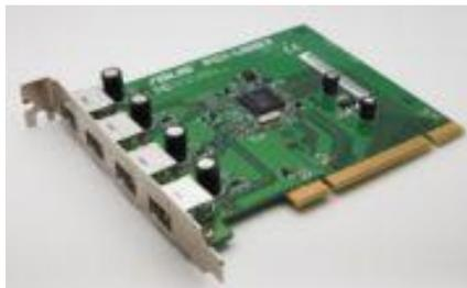
**Figura 1. 13 Tarjeta PCI-USB 2.0.**
