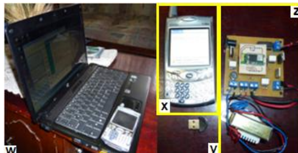
Figura 2.15 PC, PDA, Adaptador Bluetooth USB, Módulo Receptor Bluetooth
