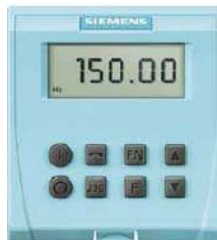
Figura 3. 4 BOP (Basic Operator Panel)
