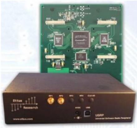
Fig. 2. Universal Software Radio Peripheral.
