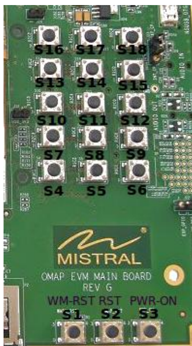
Figura. 3.14. EVM OMAP35x Main Board Push Buttons
