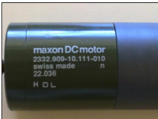
Figura2.2: Motor DC Maxon
