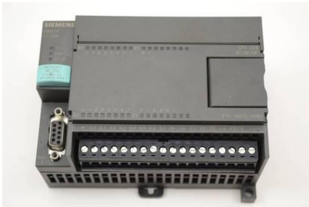
Figura 1.18. Vista Frontal de PLC SIMATIC S7 200 CPU 224 SIEMENS
