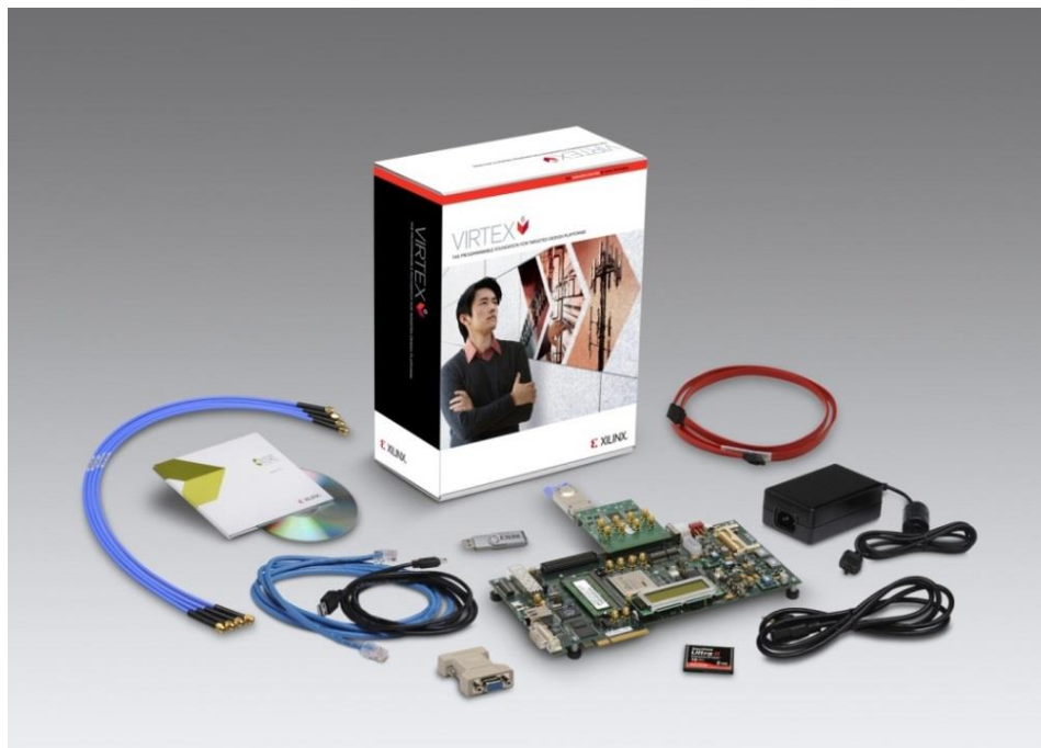
Figura. 3.7. Embedded Development Kit de Xilinx
