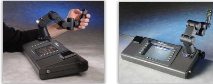
Figura 1.13: Brazo Maestro Mini-master.
