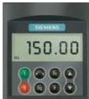
Figura 3. 4: BOP (Basic Operator Panel).
