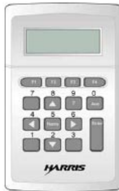
Figura. 5.14. Hand-held Terminal Unit
