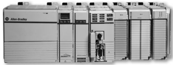
Fig. 5. PLC Allen Bradley 1768-L43
