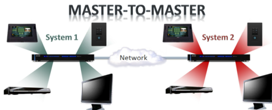
Figura 38: Sistema de control maestro a maestro (AMX Control System Expert, p. 98)
