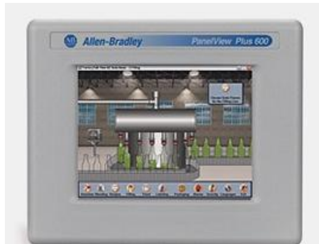
Figura 1.7: PanelView Plus de Allen Bradley.
