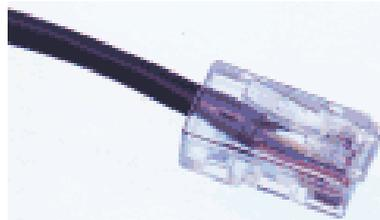
Fig 2.1 Connector RJ11
