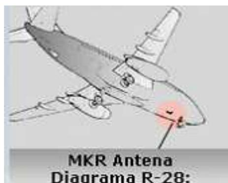
Fig.2.8 Antena Marker Beacon
