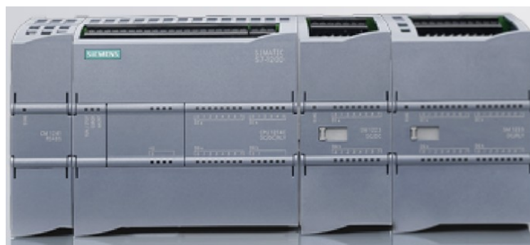
Figura 1.20 Micro PLC SIMATIC S7-1200.
