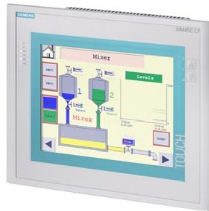
Figura 1.24 PLC Completo SIMATIC C7 - 636 TOUCH.
