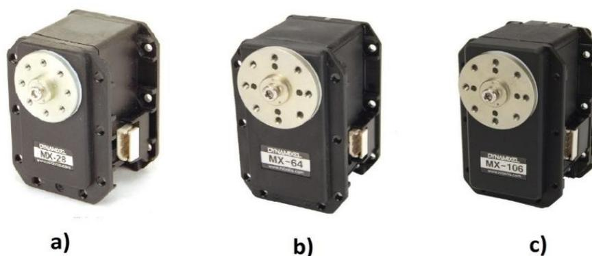
**Figura 2. 1.-** Servos Dynamixel; a) MX-28; b) MX-64; c) MX-106
