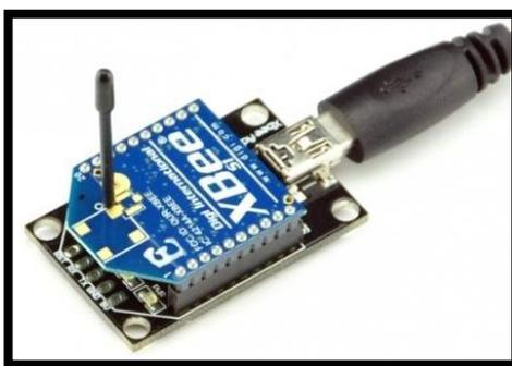
**Figura 4. 9. XBee explorer**
