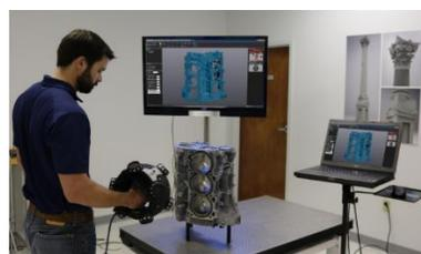
(d) Creaform Metra SCAN optically tracked 3D scanning and probing system.
