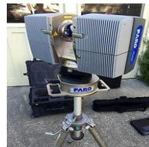
(f) Faro Photon 120 LS 3D Laser Scanner
