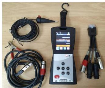
**Figura 23.** MGT-300 EVO RPM Counter
