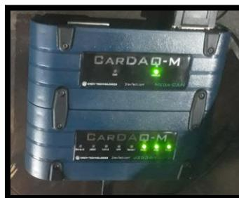
**Figura 128.** Interface Cardaq M Mega CAN
