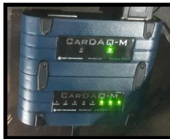
**Figura 97.** Interface Cardaq M Mega CAN
