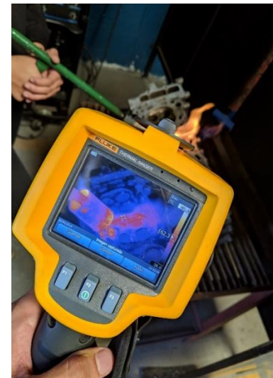
Using infrared camera
