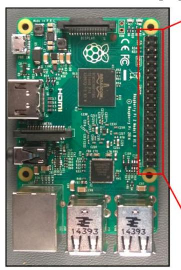
**5V PWR** I2C1 SDA 3 **5V PWR** I2C1 SCI GND GPIO 4 **UARTO TX UARTO RX** GND **GPIO 17 GPIO 18** 13 GND **GPIO 27** . GPIO 22 GPIO 23 -17 **GPIO 24** SPIO MOSI 19 **20 GND** SPIO MISO 21 GPIO 25 SPIO CSO SPIO SCLK GND SPIO CS1 28 Reserved Reserved 30 GND GPIO 5 -GPIO 12 GPIO 6 **GPIO 13** GND 35 **GPIO 19 GPIO 16 GPIO 20** GPIO 26 GND **GPIO 21**
